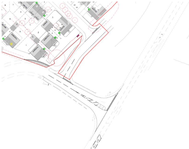
Proposed Highways Access Arrangement (Sidings Lane)
