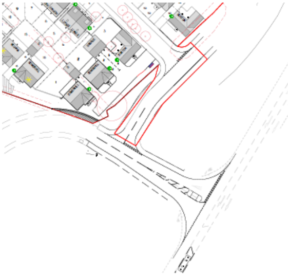
Proposed Highways Access Arrangement (Sidings Lane)
